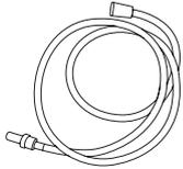
Thanks to the external hose with quick coupler, you can draw water from external sources.
