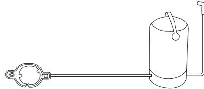
The bag was primarily designed as part of the camping kit Nestbox Tramp, but can also be used separately. The 12-liter bag and pressure showerhead are used for basic hygiene, rinsing things or washing camping cookware. The advantage is that you need no electricity to operate and you do not have to hang the shower! Thanks to the pump, the water is under pressure even when placed on the ground or inserted in the body of the kit.
